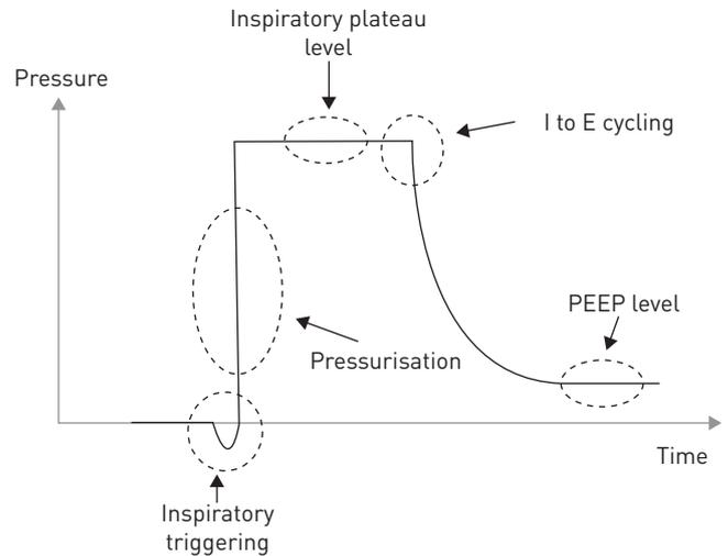
FIGURE 1 The ventilatory cycle as seen from a mask pressure-time tracing. I to E: inspiratory to expiratory; PEEP: positive end-expiratory pressure.
