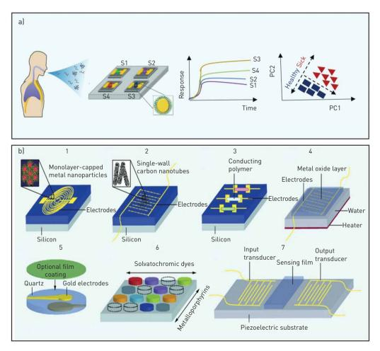
FIGURE 1 a) Overview of the working principal of nanomaterial-based sensors array. b) Different nanomaterial-based sensors. 1) Chemiresistor based on monolayer-capped nanoparticles; 2) chemiresistors based on single-wall carbon nanotubes; 3) chemiresistor based on conducting polymers; 4) chemiresistor based on metal oxide film; 5) quartz microbalance with selective coating; 6) colorimetric sensor; and 7) surface acoustic wave sensor. Reproduced from [11] with permission from the publisher.
